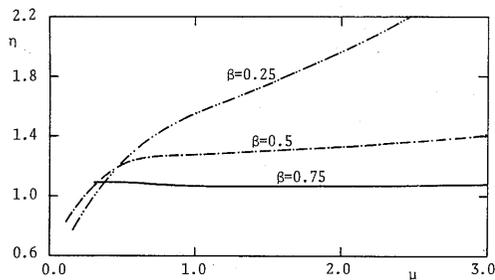
Fig. 6 Second non-dimensional frequency vs. aspect ratio: case III for  $\beta=0.25, 0.50$  and  $0.75$ .
