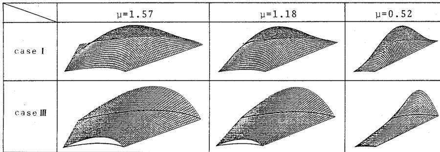
Fig. 3 Modal shapes of the annular sector plate: case I and III for  $\beta=0.5$ .
