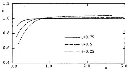
Fig. 4 First non-dimensional frequency vs. aspect ratio: case I for  $\beta=0.25, 0.50$  and  $0.75$ .
