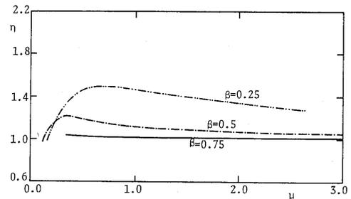
Fig. 7 Third non-dimensional frequency vs. aspect ratio: case III for  $\beta=0.25, 0.50$  and  $0.75$ .
