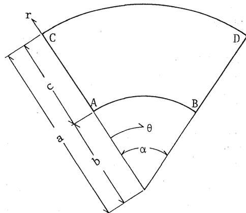
Fig. 1 Geometry of an annular sector plate.
