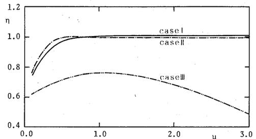
Fig. 2 First non-dimensional frequency vs. aspect ratio: case I, II and III for  $\beta=0.5$ .
