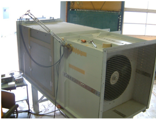
Fig. 4 Measurement method of internal flow in the inclined plane
