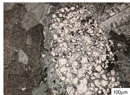
Fig. 9 Microstructure of a fragmented granule of the inoculant.
