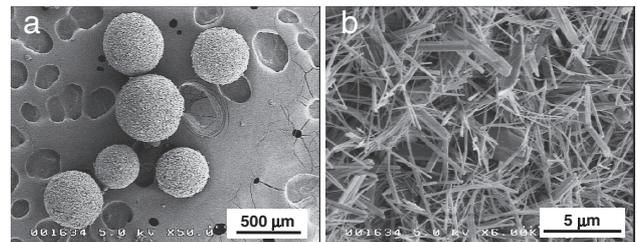
Fig. 4. SEM photographs of spherical  $\beta$ -TCP granules used in this study. Overview (a) and microstructure (b). Microstructure shows unique rod-shaped particles of  $\beta$ -TCP prepared via a hydrothermal route.
