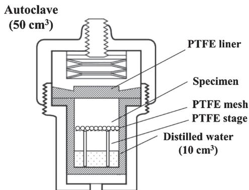
Fig. 1. Schematic illustration of apparatus for hydrothermal treatment.
