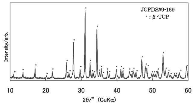
Fig. 3. XRD pattern of spherical  $\beta$ -TCP granules used in this study.
