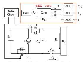
Fig. 6. Proposed digital control circuit configuration.
