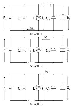
Fig.2 Equivalent circuits of charge mode.
