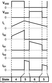
Fig. 5. Theoretical waveforms of discharge mode.
