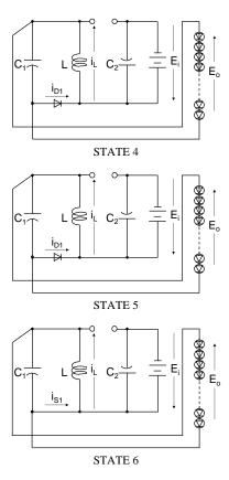
Fig. 4. Equivalent circuits of discharge mode.
