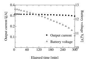
Fig. 8 Output current to LEDs, and battery voltage
