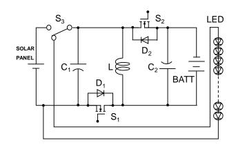
Fig.1 Proposed bidirectional DC-DC converter
