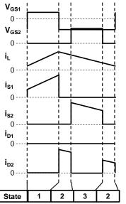
Fig.3. Theoretical waveforms of charge mode.
