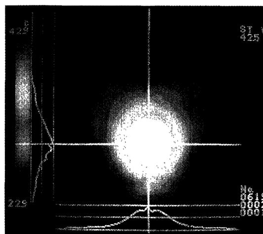
Fig. 3 Thermogram along the sagittal plane of a skull phantom after RF heating by an electrode placed at the center of the phantom. The bell-like curve (*bottom*) shows the temperature profile.
