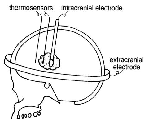
Fig. 2 Interstitial RF hyperthermia system for brain tumor. The intracranial electrode and thermocouple microprobes are implanted in the cranial cavity, and the extracranial electrode fixed over the cranium.
