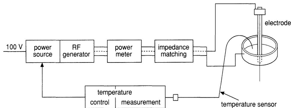
Fig. 1 Block diagram of the interstitial RF hyperthermia system, applying energy from an RF source to an external extracranial electrode and a small intracranial electrode.
