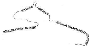
Fig. 1. Schematic representation of chemical structure of segmented polyurethanes.
