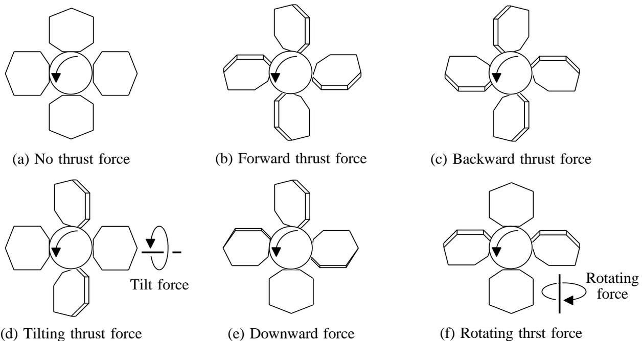
Fig. 5 Functions of VARIVEC Propeller (rear view of AUV)
