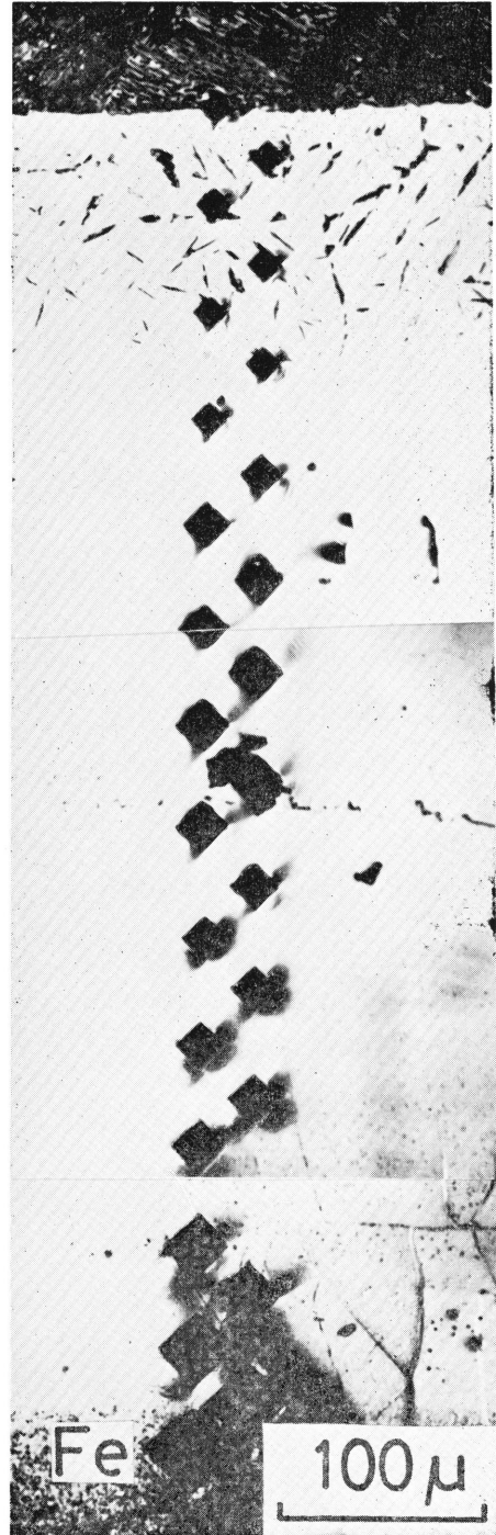
Photo. 2 Structure of diffused layer ( 1100^{\circ}\text{C}\times 20\text{hr} )
