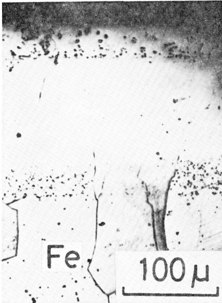
Photo. 1 Structure of diffused layer ( 900^{\circ}\text{C}\times 20\text{hr} )
