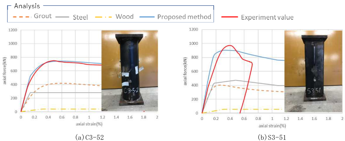
Fig. 4 Relations between axial force and axial strain of test and analysis
