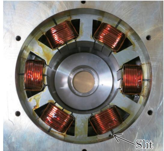
Fig. 9. The stator of the prototype.
