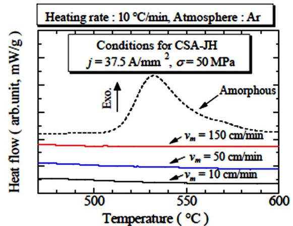
FIG. 2. (Color online) DSC curves of ribbons prepared under the varied moving velocities of 10, 50, and 150 cm/min. The measurement was carried out in a temperature range from 480 to 600 °C, and the heating rate was fixed at 10 °C/min.
