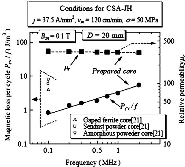
FIG. 4. Relative permeability  $\mu_r$  and magnetic loss per cycle  $P_{cv}/f$  of a developed core as a function of frequency, together with those for different types of cores with controlled permeability (Ref. 21).
