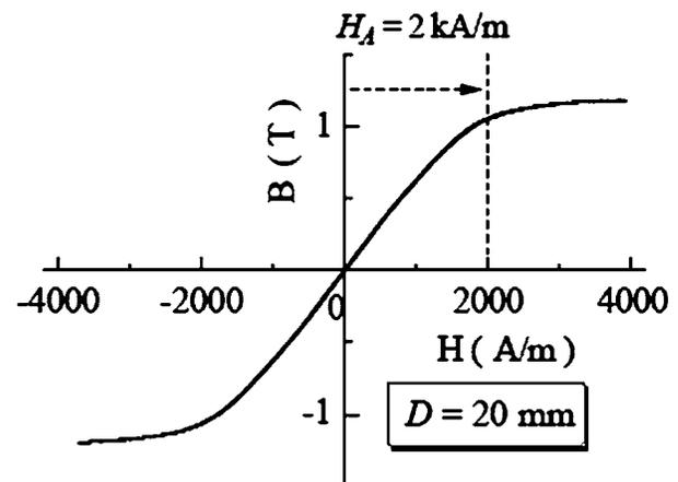
FIG. 3. dc hysteresis loop of a prepared core made from a 500-mm-long ribbon. The long ribbon was fabricated by high speed CSA-JH method ( $j = 37.5 \text{ A/mm}^2$ ,  $v_m = 120 \text{ cm/min}$ , and  $\sigma = 50 \text{ MPa}$ ).
