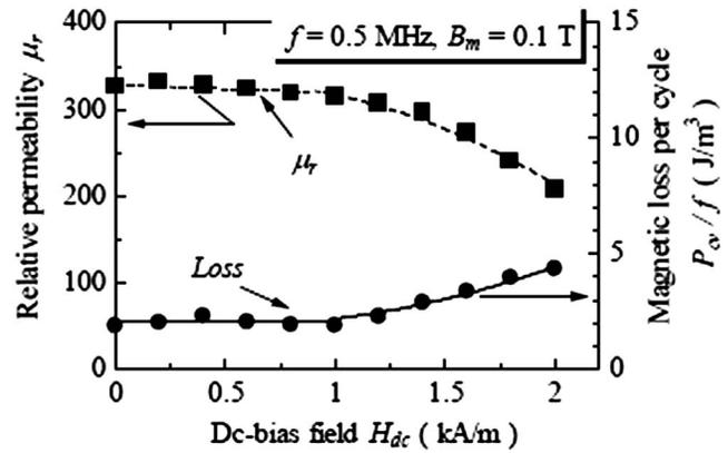
FIG. 5. Dependence of relative permeability  $\mu_r$  and magnetic loss per cycle  $P_{cv}/f$  on dc-bias field,  $H_{dc}$ . The measurement was carried out at  $f = 0.5$  MHz and  $B_m = 0.1$  T.
