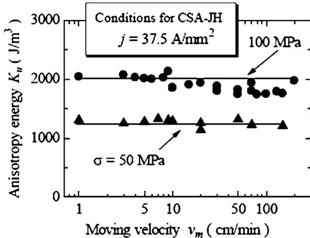
FIG. 1. Anisotropy energy  $K_u$  of ribbons prepared by continuous stress-annealing by Joule heating (CSA-JH) as a function of moving velocity  $v_m$ . The current density  $j$  was set at  $37.5 \text{ A/mm}^2$ . The ribbons were annealed under the tensile stress of 50 or 100 MPa.
