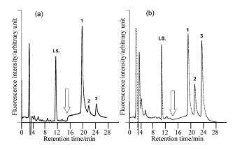
Fig. 2 Chromatograms of a standard solution (a) and turmeric powder G (b). The peak number: 1, BDMC; 2, DMC; 3, C. The arrow indicates changing of the detection wavelengths from 287 nm ( $\lambda_{ex}$ ) and 303 nm ( $\lambda_{em}$ ) for I.S. to 426 nm ( $\lambda_{ex}$ ) and 539 nm ( $\lambda_{em}$ ) for curcuminoids.
