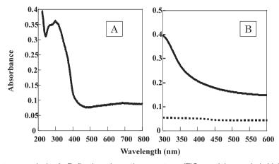
**Fig. 3** Absorption spectrum analysis. A: Reflection absorption spectrum (TiO<sub>2</sub> particle powder). Light absorption bands are present in the visible light range at 400 nm and above. B: Transmission absorption spectrum (TiO<sub>2</sub> particle mixture). The TiO<sub>2</sub> particle mixture (solid line, 5 mg/mL concentration) shows higher active wavelengths, extending into the visible range, than pure water (dotted line).
