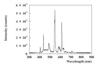
Fig. 1 Fluorescent light wavelength. Wavelength is measured at a distance of 5 cm; the same distance used in the experiment. The luminous intensity is almost 300 lux. The light itself contains no UV rays.
