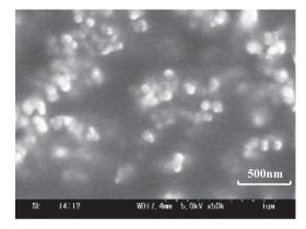
Fig. 2 SEM images of  $TiO_2$  particles in the aqueous mixture. Aggregates approximately 100 nm in diameter are well dispersed among the primary particles. Scale bar = 500 nm
