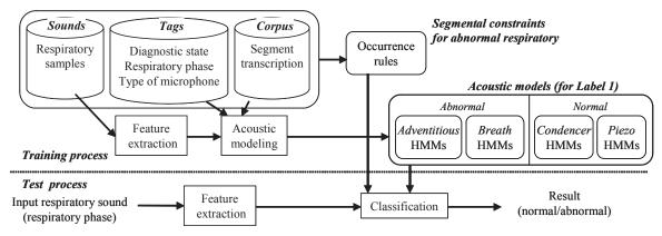
Figure 3: Architecture of classification system between normal and abnormal respiratory
