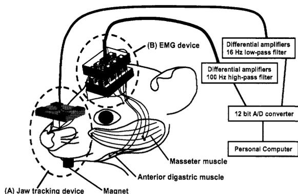
Fig. 1 Block diagram of the recording system. The recording system consists of (A) jaw tracking device and (B) EMG device. The jaw movement and EMG signals are stored simultaneously in computer memory.
