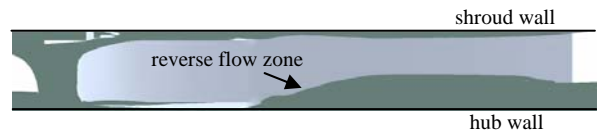
Fig.8 Reverse flow zone (with both grooves, \phi=0.13 )
