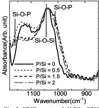
Fig. 2. FT-IR spectra of  $H_3PO_4$  :E201 membranes with different P/Si ratio.
