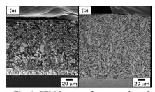
Fig. 1. SEM images of cross-section of Cs-PWA-dispersed membranes, which employed (a) Epicoat 828 and (b) E201 as matrices.
