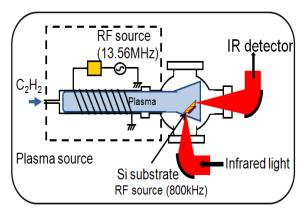
and the thickness after the deposition measured with the profilemeter. Plasma was generated by 13.56 MHz RF power. The substrate bias was fed by 800kHz RF power.
