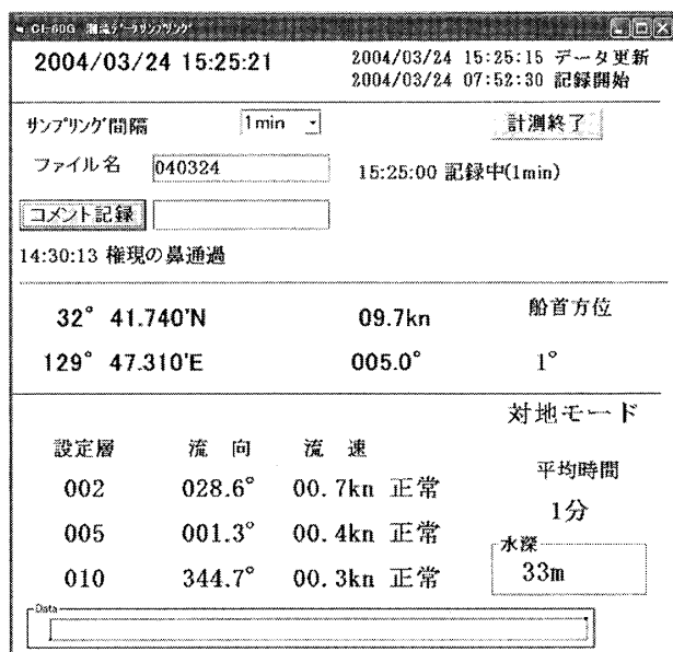
Fig. 10 Example screen of acquisition of the tidal current data by R.V. Kakusui.
