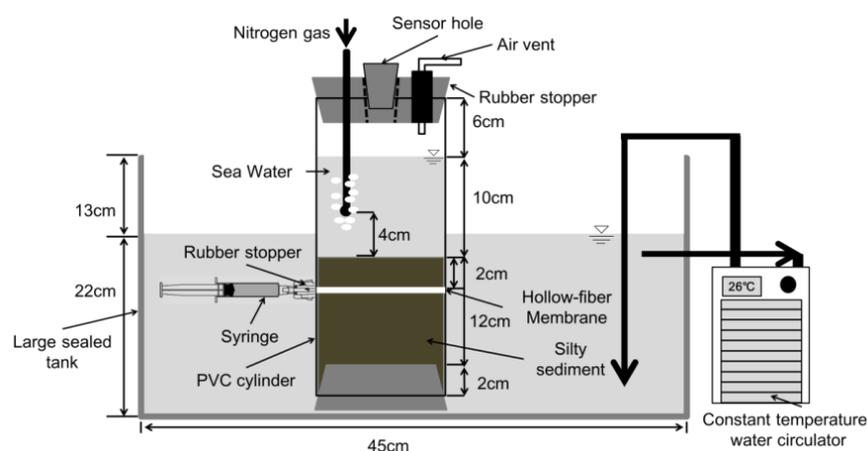
Figure 5-1 Schematic figure of the equipment for incubation experiment. Control group (no addition group) and  $\text{Mg}(\text{OH})_2$ , NaOH,  $\text{MgCl}_2$  addition groups were set up. Chemical reagent ( $\text{Mg}(\text{OH})_2$ , NaOH and  $\text{MgCl}_2 \cdot 6\text{H}_2\text{O}$ ) were mixed well with sediments before transferred into
