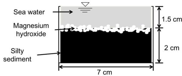
Figure 3-1 Magnesium hydroxide ( $Mg(OH)_2$ ) capping on silty sediments
