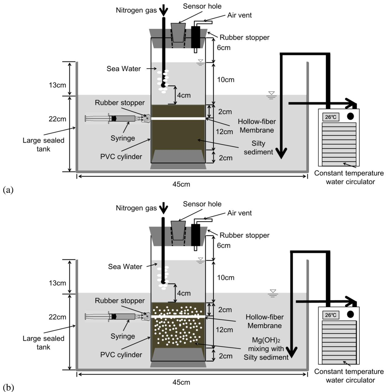
Figure 3-3 Schematic figure of the equipment for Experiment-2. (a) Control group without  $Mg(OH)_2$ , (b) Treatment group with  $Mg(OH)_2$  granules mixed in the sediments
