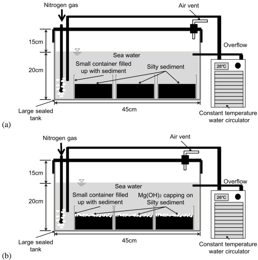
Figure 3-2 Schematic figure of the equipment for Experiment-1. (a) Control group without  $Mg(OH)_2$ , (b) Treatment group with  $Mg(OH)_2$  granules scattered on the sediments
