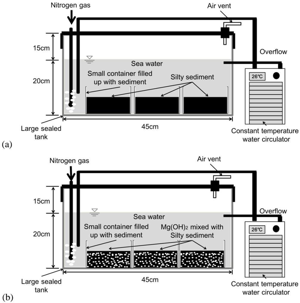
Figure 4-2 Schematic figure of the equipment for Experiment-1. (a) Control group without  $Mg(OH)_2$ , (b) Treatment group with  $Mg(OH)_2$  granules scattered on the sediments
