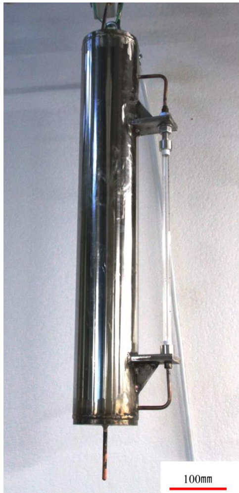
Fig.2.39 Appearance photo of deaeration water generation tank
