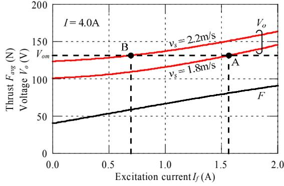
Fig. 4. Effects of  $I_f$  on the thrust and the voltage.
