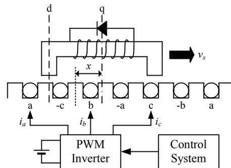
Fig.1. Structure of the novel LSM.
