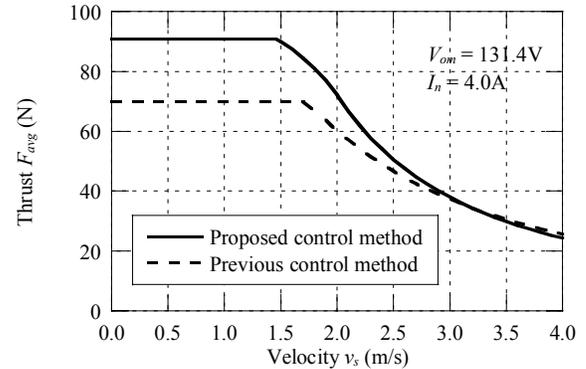
Fig. 8. Comparison of the thrust characteristics of the proposed control method with that of the previous control method.
