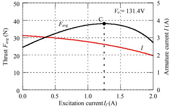
Fig. 6. Effects of  $I_f$  on the thrust and the armature current.
