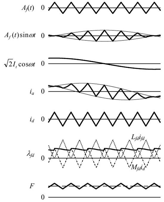
Fig. 3. Current, flux, and thrust waveform.
