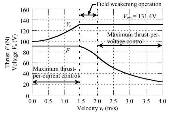
(a) Thrust and voltage characteristics.
