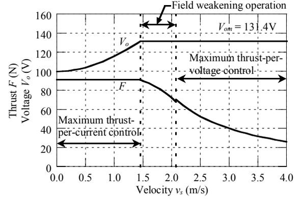
(a) Thrust and voltage characteristics.
