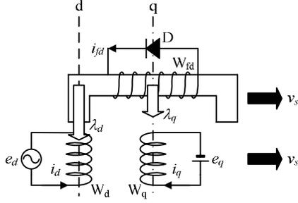
Fig. 2. Equivalent model on the dq-axis.
