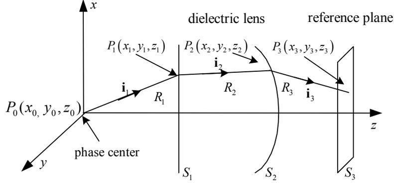
Figure 1. Coordinate system for ray tracing method
