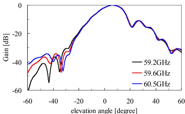
Figure 5. The variation of electric field radiation pattern
