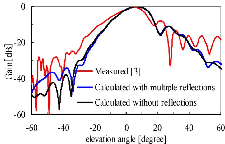
Figure 4. The electric field radiation pattern
