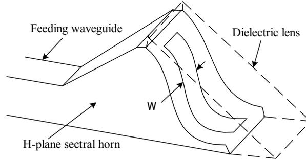
Figure 2. Geometry of dielectric lens antenna
