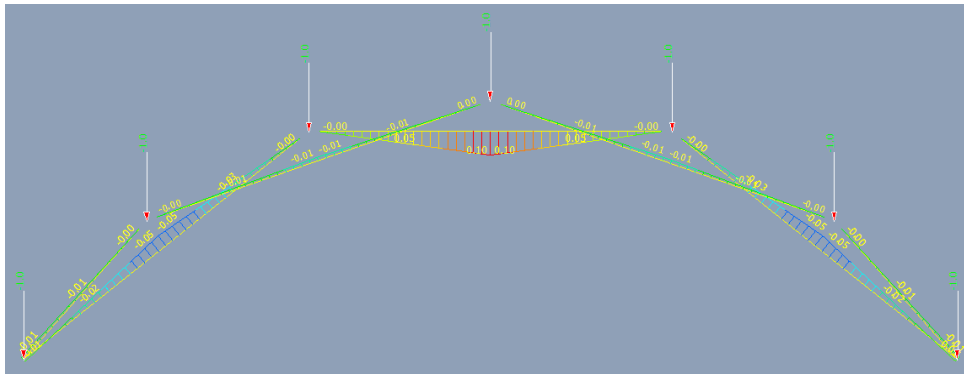
Fig. 7-19 Bending moment of the main arch structure
