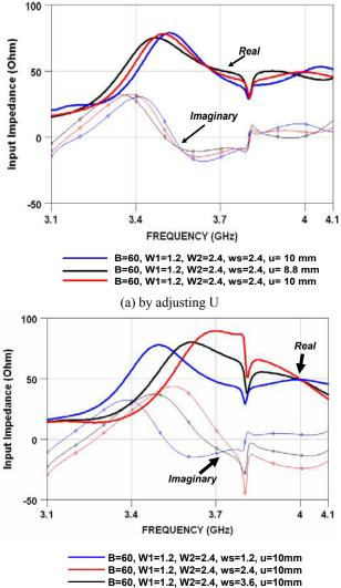
(b) by adjusting ws Figure 9 The Input Impedance Characteristics
