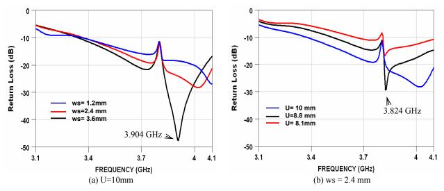
Figure 4. Return loss characteristics. B = 60 mm, W1 = 1.2 mm, W2 = 2.4 mm, g = 0.2 mm
