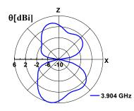
Figure 6 Electric field radiation characteristics at 3.904 GHz B = 60 mm, W1 = 1.2 mm, W2 = 2.4 mm, L1 = 11.2 mm, L2 = 10.5 mm, ws = 3.6 mm, g = 0.2 mm, U = 10 mm.
