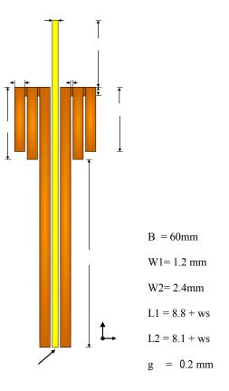
Figure 1 Structure of planar sleeve antenna
