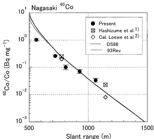
**Fig. 3.** Specific  $^{60}\text{Co}$  activity (at the time of the explosion) as a function of the slant range. Data were taken by Hashizume *et al.*<sup>1)</sup> for steel bars 8 cm depth in concrete. A corresponding calculation by Loewe *et al.*<sup>2)</sup> is also shown. The solid and dotted lines indicate the activation calculation in a free field in air.
