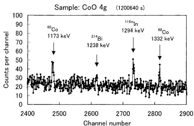
**Fig. 4.** Gamma-ray spectra of cobalt activation by environmental neutrons. The sample was four grams of CoO.
