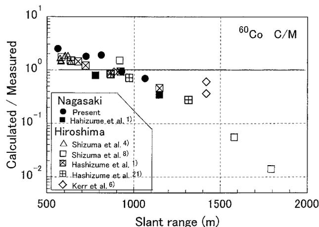
Fig. 5. Comparison of the C/M ratios of  $^{60}\text{Co}$  for Nagasaki and Hiroshima.
