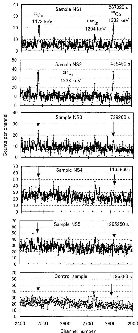
**Fig. 2.** Partial spectra around the 1173 and the 1332 keV gamma rays from  $^{60}\text{Co}$  for steel samples. Takatani house (GR = 290 m), Shiroyama School (GR = 540 m), Nagasaki University Hospital (GR = 653 m), Motoki Bridge (GR = 780 m), Mitsubishi Steel (GR = 935 m), and a control sample<sup>8)</sup> of Army Food storehouse in Hiroshima.
