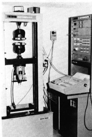
**Fig. 1.** Showing tensile meter, DSC 500 (SHIMAZU CO.) Left half measuring the tensile strength and right half was recording parts.
