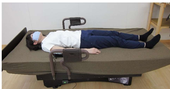
Figure 1. An electric sway bed (dimensions: 1900 × 900 × 500 mm (length × width × height)), powered by an electric motor, with seven sway speed settings. The motorized device was set to sway the student vertically by ±2 cm for a total of 4 cm. In this study, the level 2 (0.64 Hz) sway speed was used.
