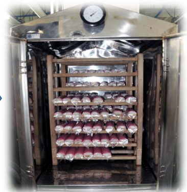
Two stage heating Step of first heating : 40°C Step of second heating : 90°C
