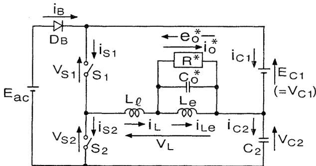
Fig. 2 Simplified equivalent circuit of Fig.1.
