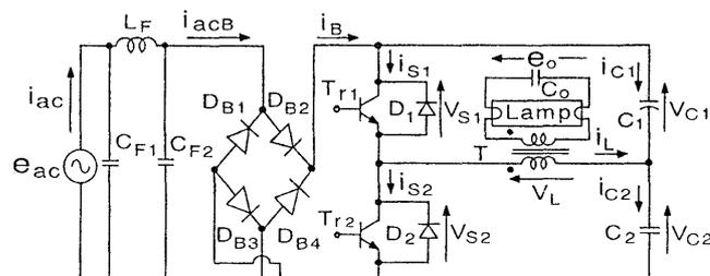
Fig. 1 Basic circuit configuration of the new modified half-bridge type inverter for the electronic ballast of fluorescent lamps.
