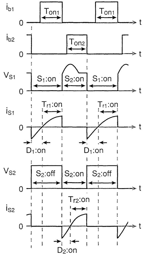
Fig. 3 Typical waveforms of the driving base currents  $i_{b1}$  and  $i_{b2}$  of  $T_{r1}$  and  $T_{r2}$ , respectively, voltage  $V_{S1}$  and current  $i_{S1}$  of  $S_1$ , and voltage  $V_{S2}$  and current  $i_{S2}$  of  $S_2$  in Fig.1 or Fig.2.
