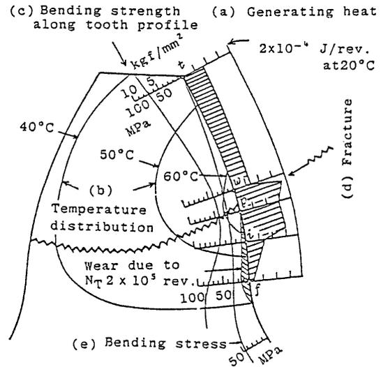
Fig.12 Generated heat, temperature distribution, tensile strength and bending stress
