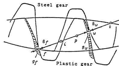
Fig.4 Load sharing ratio for worn teeth
