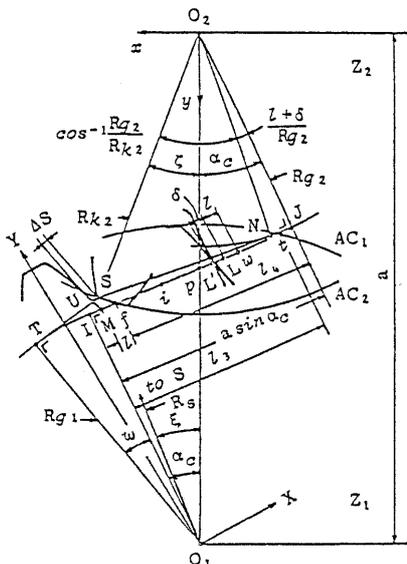
Fig.6 Interference near tooth root
