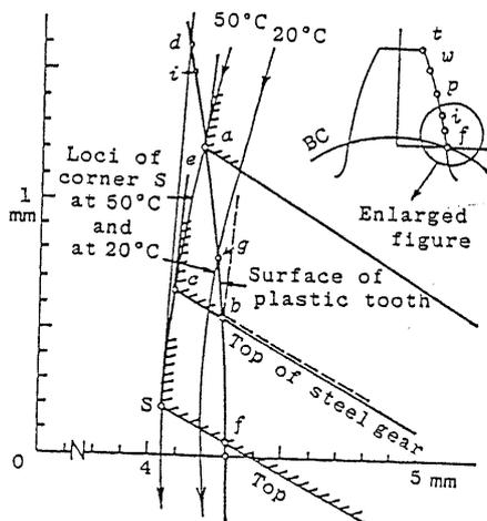
Fig.8 Scraping by tip corner of steel tooth
