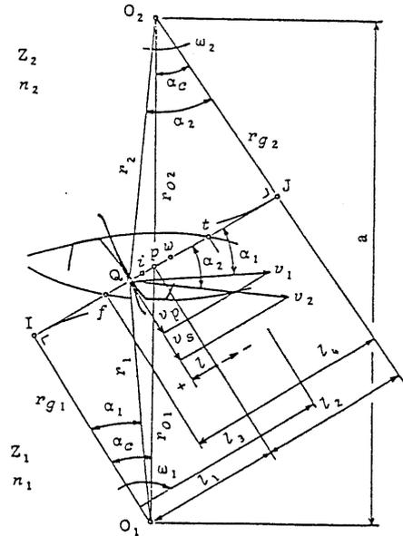
Fig.3 Sliding velocity and specific sliding
