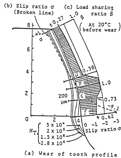
Fig.5 Wear, specific sliding and load sharing ratio
