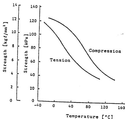
Fig.14 Strength of MC-nylon
