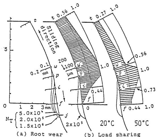
Fig.10 Abnormal wear near tooth root
