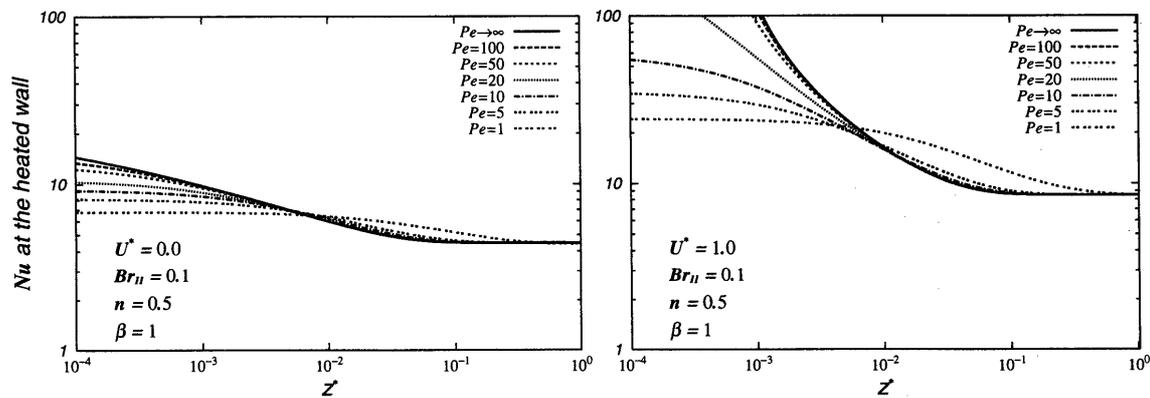
Fig. 12  $Nu$  variations with  $Pe$  for heat transfer to a pseudoplastic fluid ( $n=0.5, \beta=1$ ) with significant viscous dissipation ( $Br=0.1$ ), Case II
