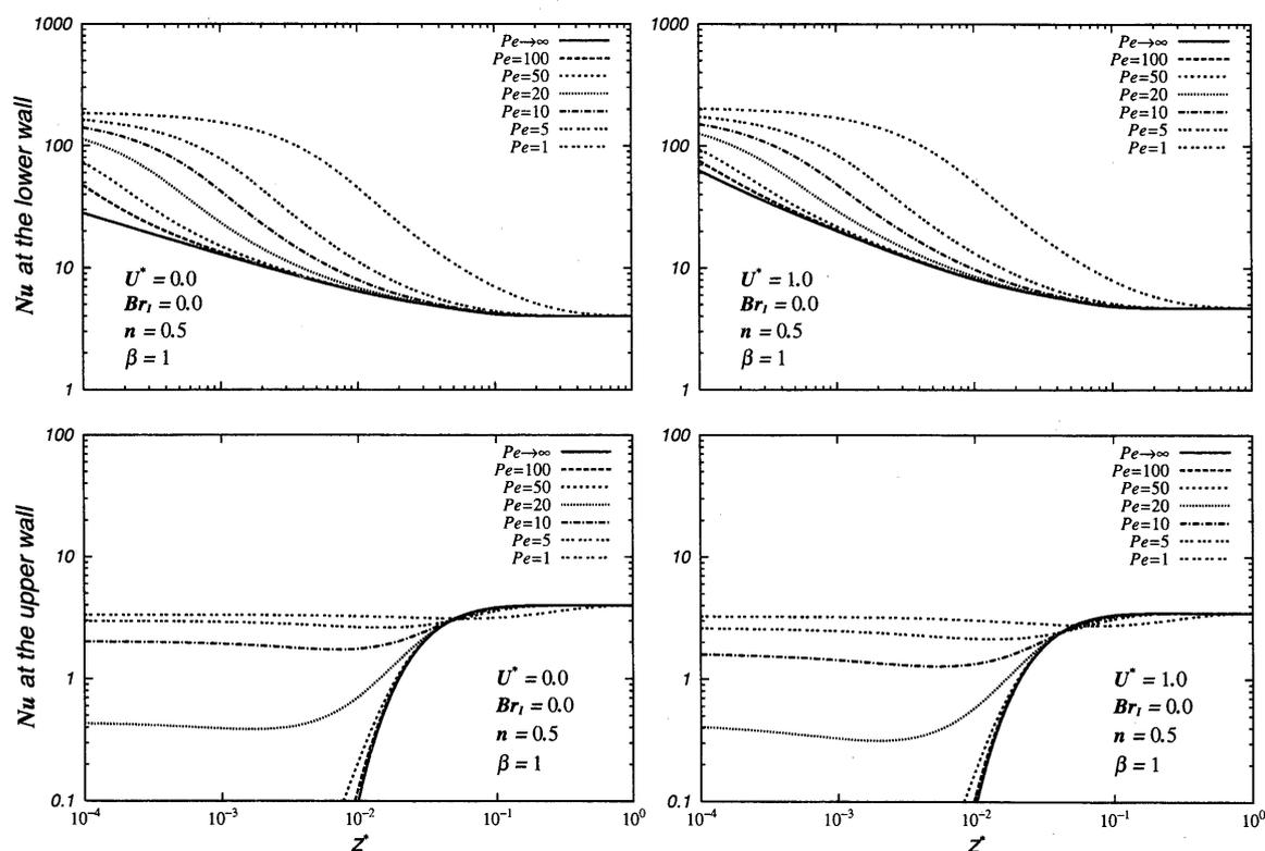
Fig. 7  $Nu$  variations with  $Pe$  for heat transfer to a pseudoplastic fluid ( $n=0.5, \beta=1$ ) without viscous dissipation ( $Br=0$ ), Case I
