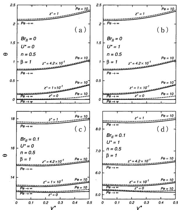
Fig. 5 Developing temperature profiles for  $U^*=0$  and  $U^*=1$  (Case II)
