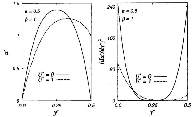
Fig. 2 Velocity profile and square of velocity gradient ( $n=0.5, \beta=1$ )
