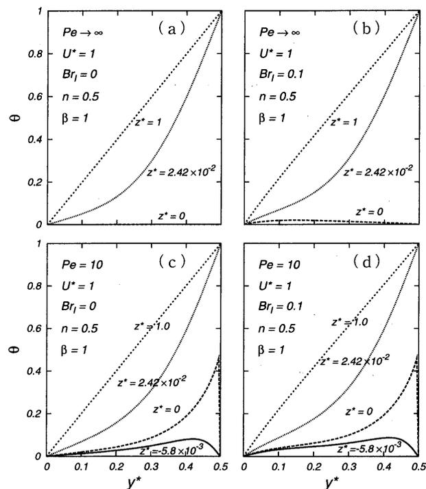
Fig. 4 Developing temperature profiles ( $U^*=1$ )
