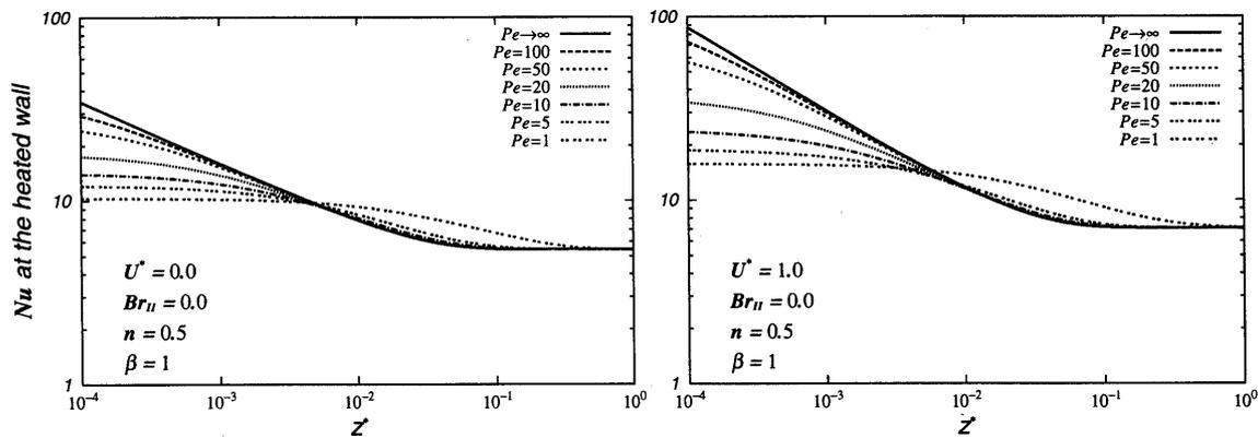
Fig. 11  $Nu$  variations with  $Pe$  for heat transfer to a pseudoplastic fluid ( $n=0.5, \beta=1$ ) without viscous dissipation ( $Br=0$ ), Case II
