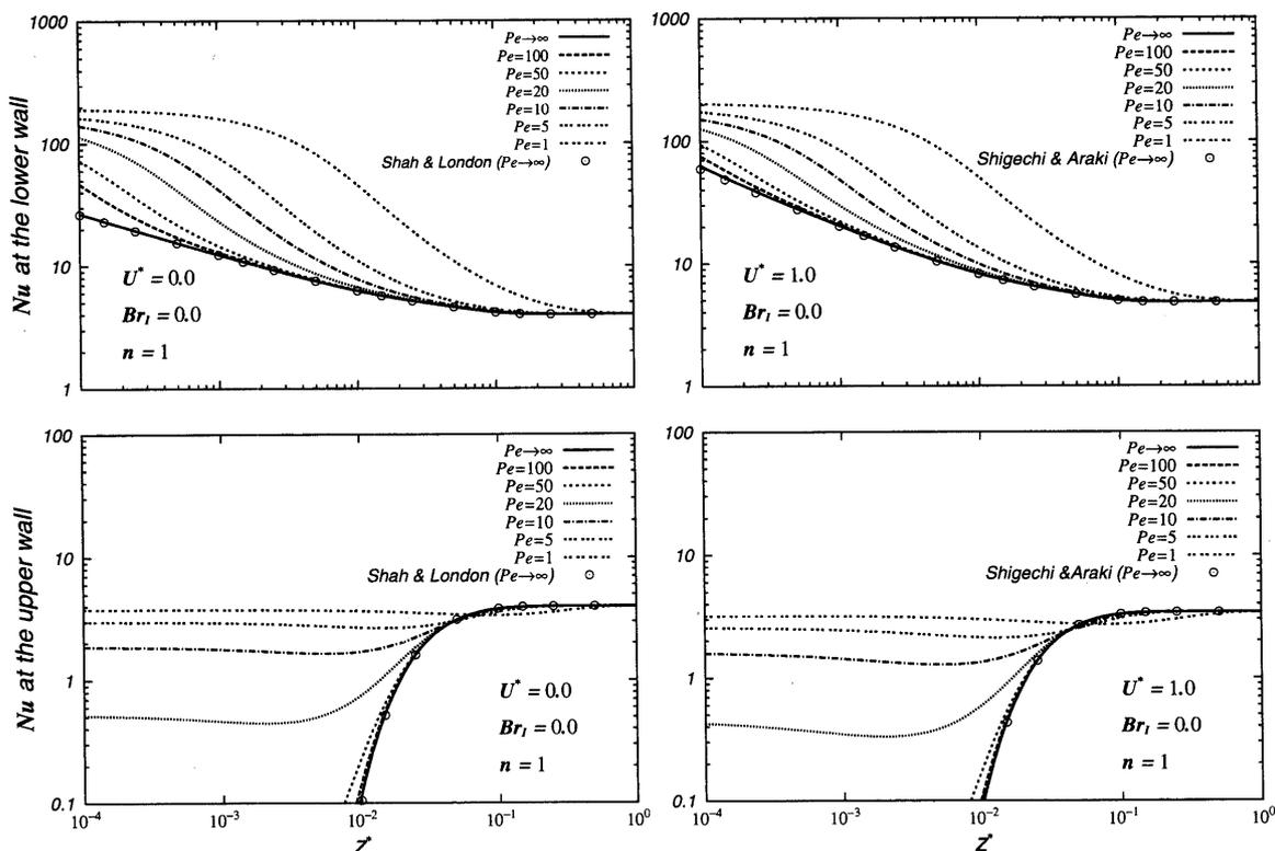
Fig. 6  $Nu$  variations with  $Pe$  for heat transfer to a Newtonian fluid ( $n=1$ ) without viscous dissipation ( $Br=0$ ), Case I
