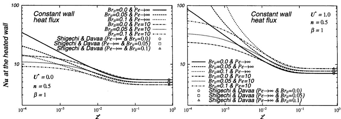
Fig. 13 Effects of  $Br$  and  $Pe$  on  $Nu$  at the walls for Case II ( $n=0.5$ ,  $\beta=1$ )
