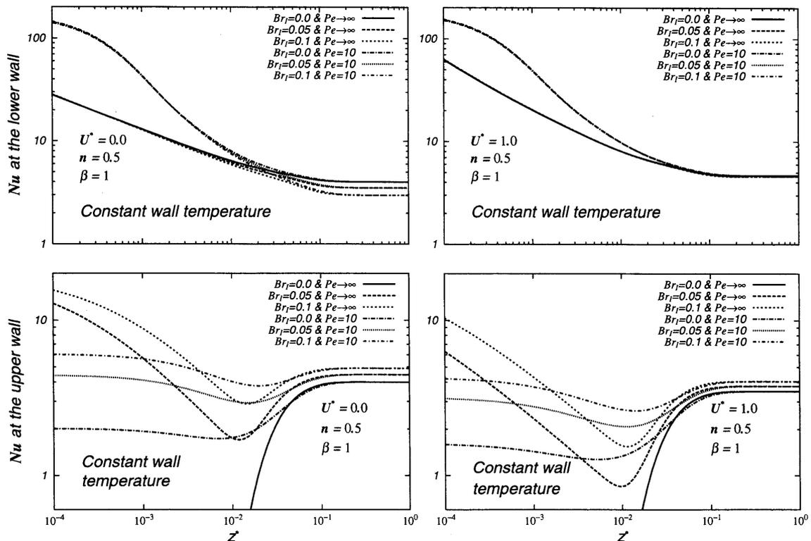
Fig. 9 Effects of  $Br$  and  $Pe$  on  $Nu$  at the walls for Case I ( $n=0.5$ ,  $\beta=1$ )
