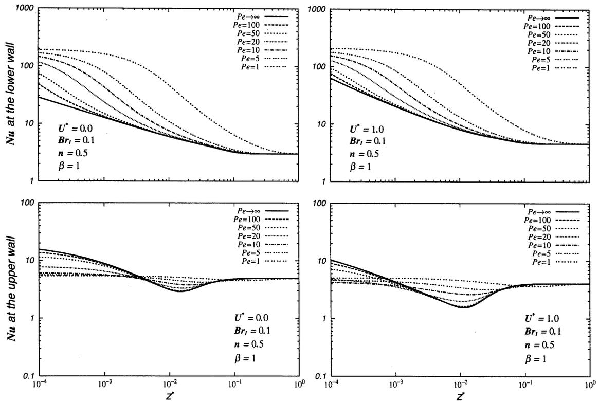
Fig. 8  $Nu$  variations with  $Pe$  for heat transfer to a pseudoplastic fluid ( $n=0.5$ ,  $\beta=1$ ) with significant viscous dissipation ( $Br=0.1$ ), Case I
