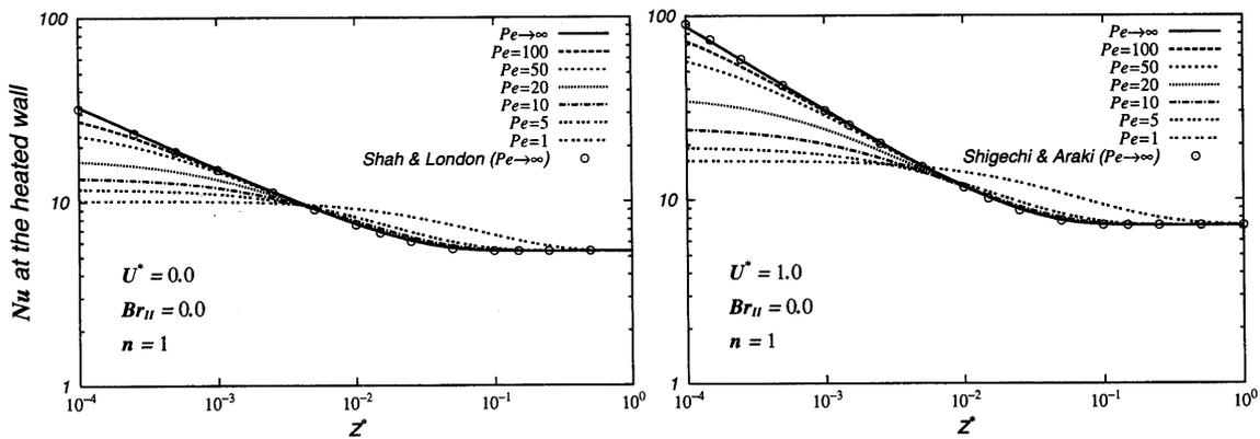
Fig. 10  $Nu$  variations with  $Pe$  for heat transfer to a Newtonian fluid ( $n=1$ ) without viscous dissipation ( $Br=0$ ), Case II
