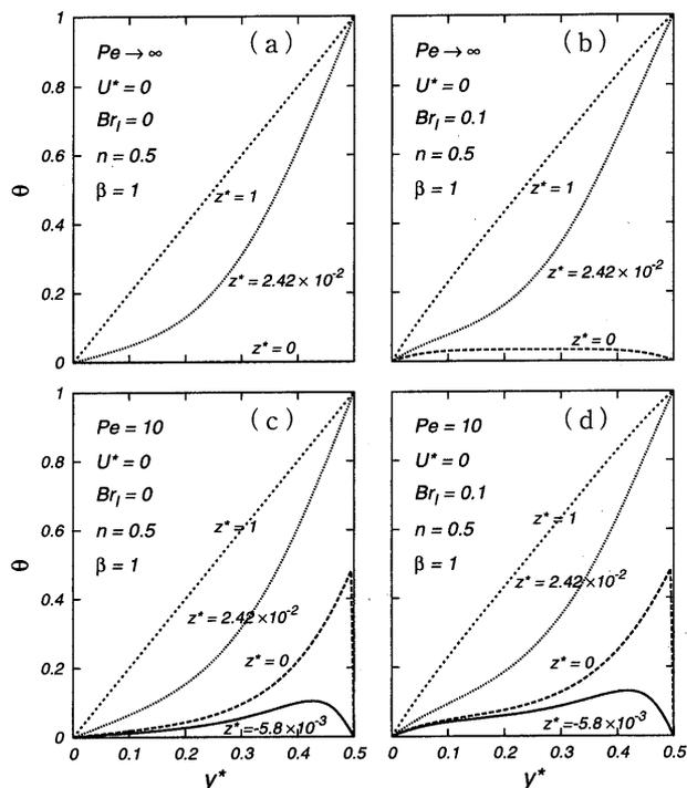
Fig. 3 Developing temperature profiles ( $U^*=0$ )
