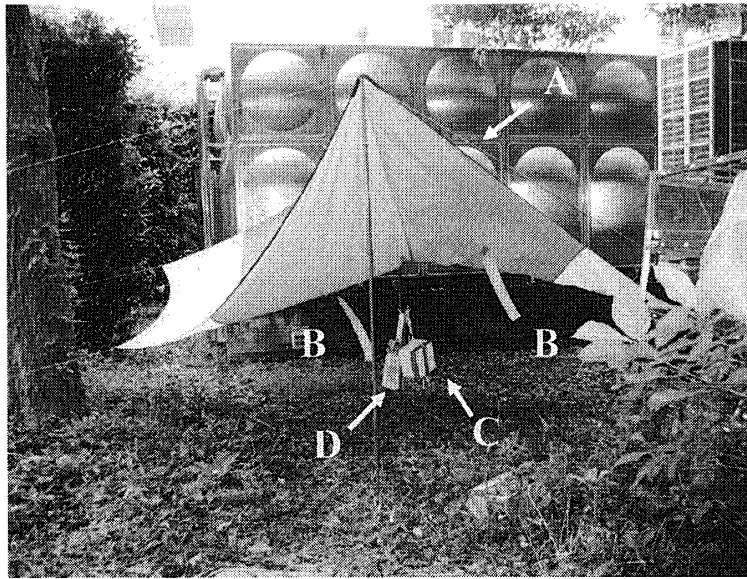
Fig. 2. Outline of field test design. A, Tarpaulin; B, Insecticide-impregnated paper strips; C, Styrofoam box containing dry ice; D, CDC-type miniature mosquito trap.
