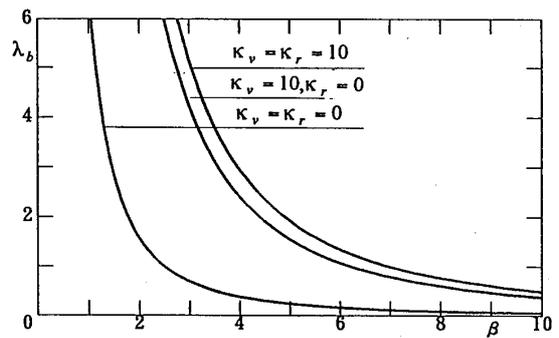
Fig. 6 Buckling curves:  $\beta^*=0.6$
