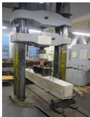
Fig. 5.9 An example of concrete beam during loading.
