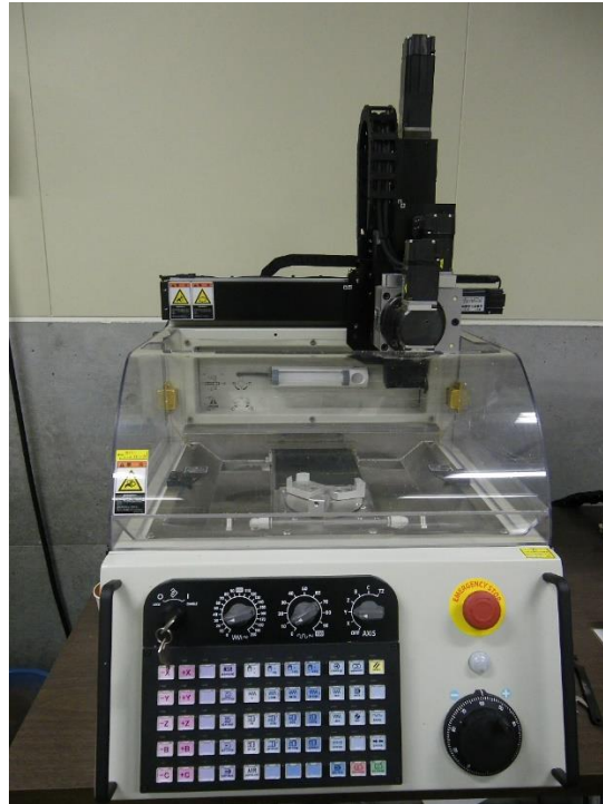
Fig. 5.7. Images of 5-axis machine tool (UNC-100-M5).
