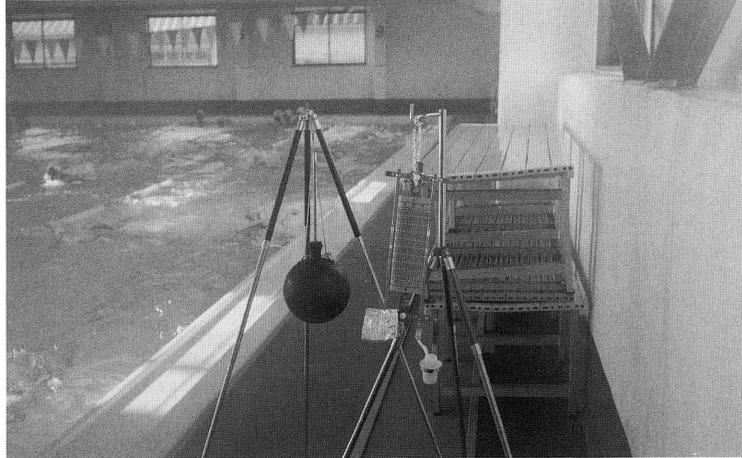
Figure 1 Environment temperature measurement apparatus.
