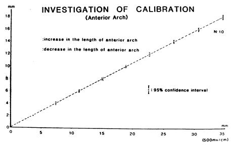
Fig. 5. A reliable linearity of the electrogoniometer A was confirmed.
