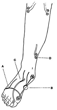
Fig. 4. Shematic picture of the fixation of the electrogoniometer A, B and C and the surface electrod of the electromyogram D.
