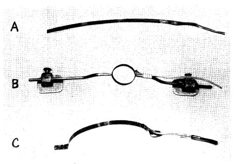
Fig. 2. The picture of the electrogoniometers A, B and C.
