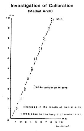
Fig. 6. A reliable linearity of the electrogoniometer B was confirmed.
