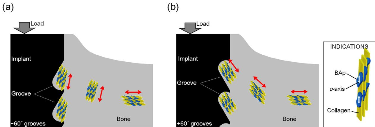
**Fig. 7.** Schematics of the preferentially aligned bone microstructure of BAp *c*-axis/collagen fibers in the case that the groove angle was (a)  $-60^\circ$  and (b)  $+60^\circ$ , reproduced based on the data in Fig. 3g, Fig. 5b, and Fig. 6b. Only in the  $+60^\circ$  groove, the direction of the BAp *c*-axis/collagen fiber alignment continuously changed from inside of the groove to the host tibia bone through the bone inside the groove.
