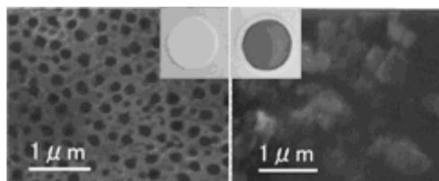
(a) AAO disc (b) After electrophoresis
