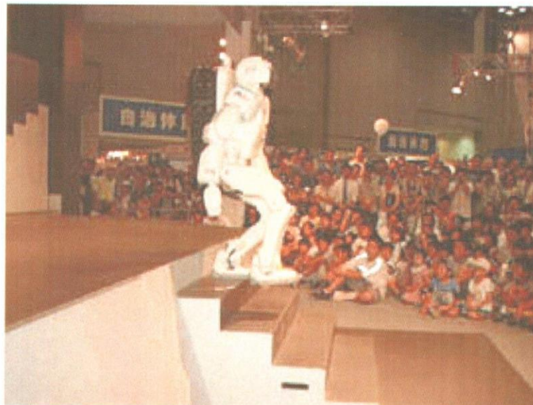
Fig. 9 Honda P3 robot negotiating stairs
