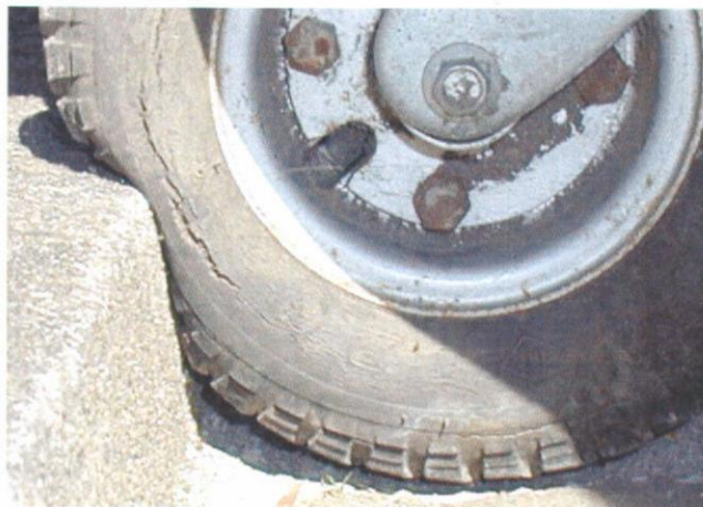
Fig. 8 Negotiation of a 7 cm curb by a 20cm diameter tire under maximum loading
