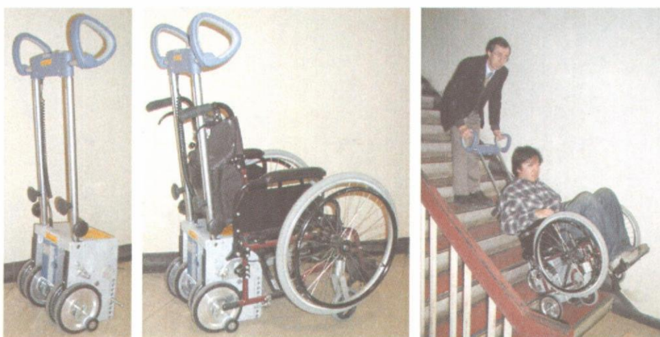
(a) Stair-climb mech. (b) Mech. attached to wheelchair (c) Stair-climbing operation
