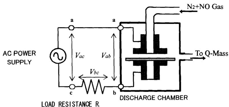
Fig.2 Experimental Circuit
