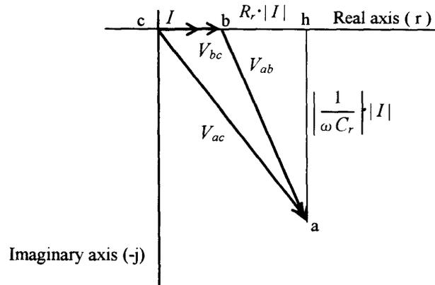
Fig.6 Vector figure of  $V_{ac}$ ,  $V_{ab}$  and  $V_{bc}$
