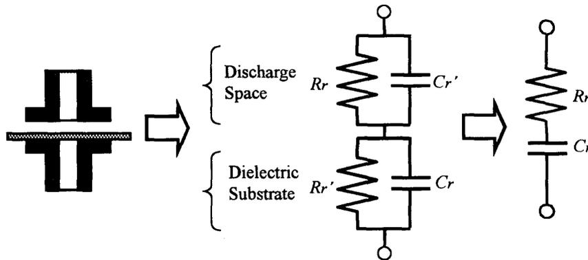
Fig.4 The equivalent circuit of barrier discharge.
