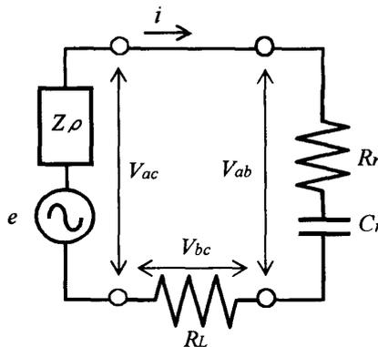
Fig.5 Equivalent circuit of reactor part
