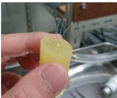
Fig. 5 Check flow condition of bundle of HF
