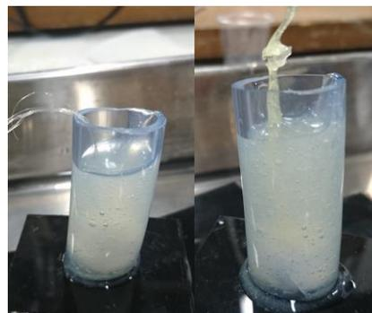
(c) Finished parts of HF( hollow fibers)
