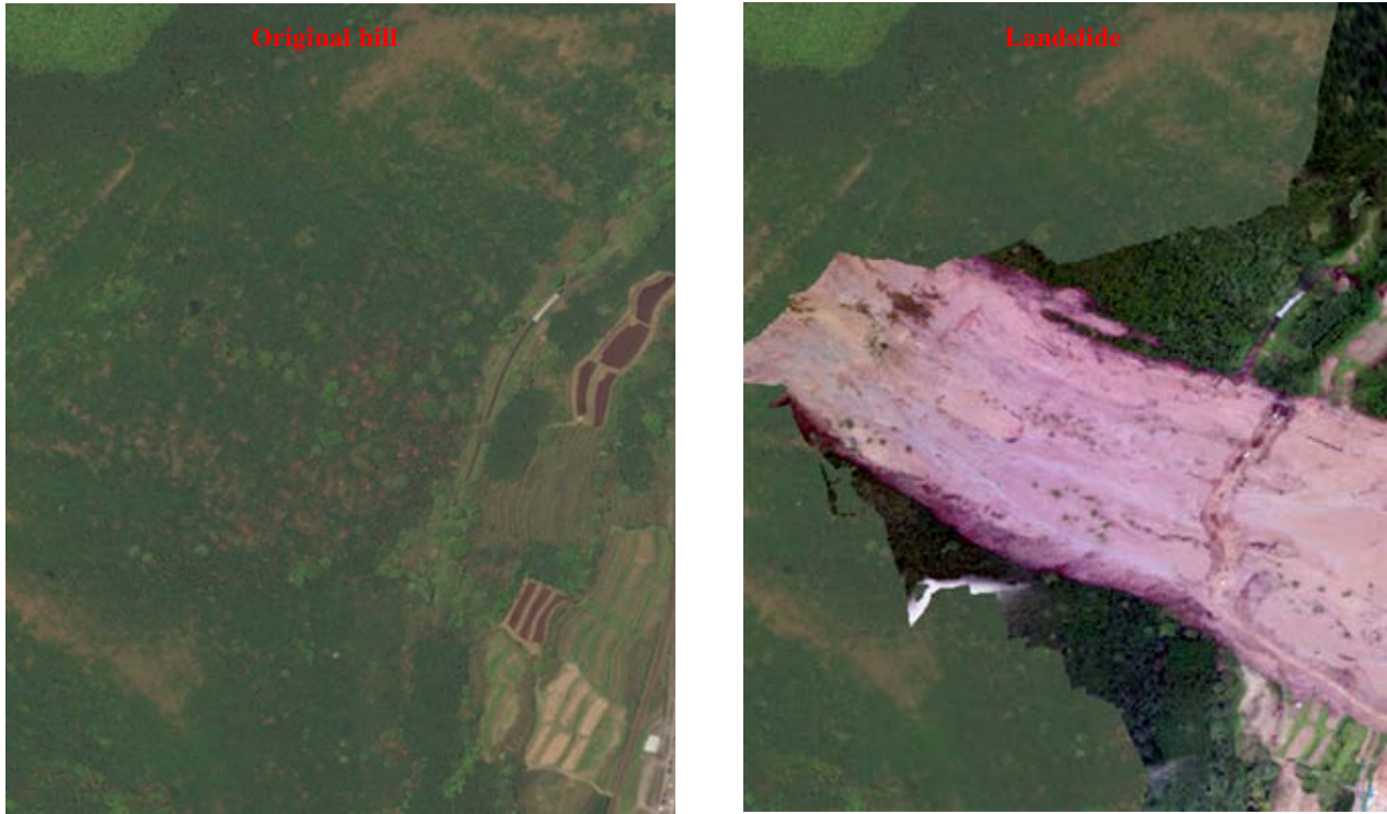
Fig. 8 West slopes of Aso Big Bridge (The original hill and after landslide).
