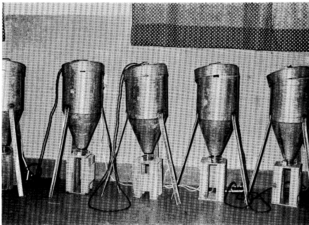
Fig. 2. Tullgren apparatus for collection of unengorged larvae from soil samples.
