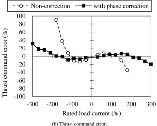
Fig. 14. Measured effect of the phase correction.
