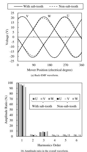
Fig. 10. Analysis of back-EMF characteristics.
