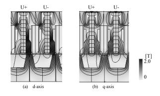
Fig. 5. Magnetic flux density distribution and line.
