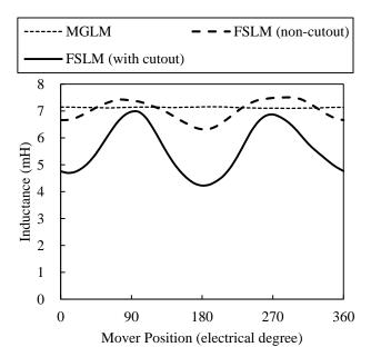
Fig. 6. Analysis of inductance characteristics (Lu, 100 coil turns).
