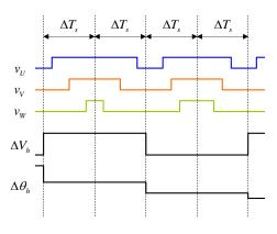
Fig. 2. Waveforms of the PWM voltage and injected voltage.
