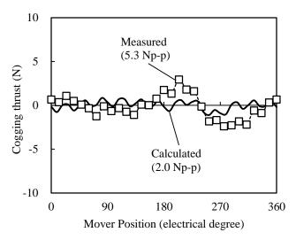
Fig. 16. Cogging thrust characteristics.
