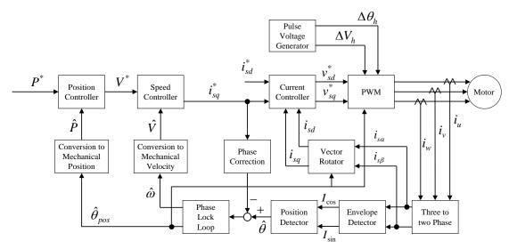
Fig. 1. Block diagram of the sensorless control.
