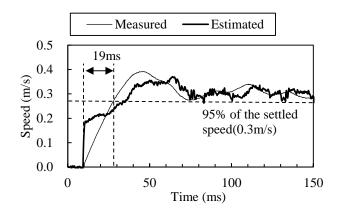
Fig. 19. Speed control dynamics characteristics.
