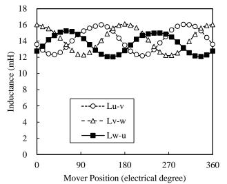
Fig. 12. Measured inductance characteristics.
