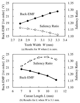
Fig. 8. Analysis of results for the saliency ratio and back-EMF.
