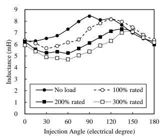
Fig. 13. Measured inductance characteristics at each rated load condition.
