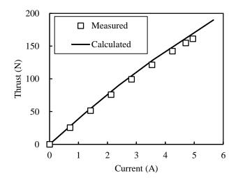
Fig. 15. Measured thrust characteristics.
