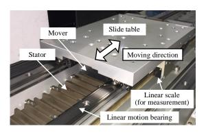
Fig. 17. Linear slider used for driving motion.
