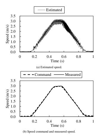
Fig. 18. Moving speed characteristics achieved by sensorless control.
