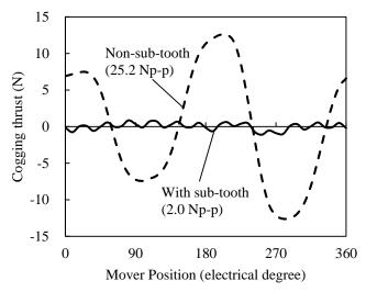
Fig. 9. Analysis of cogging thrust characteristics.
