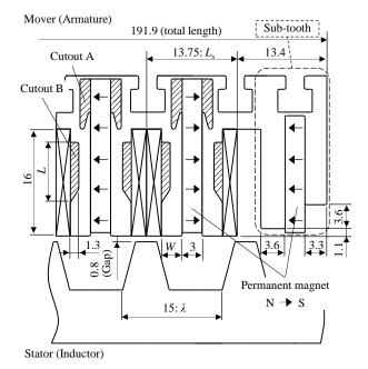
Fig. 7. Proposed schematic diagram of a FSLM. The units are mm. Hatched areas indicate the cutout in the core. The length of the laminate in the laminating direction is 50 mm.
