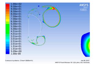
**Figure 10.** Distribution of vorticity for a semicircle at t = 18 s. Descending Cl.
