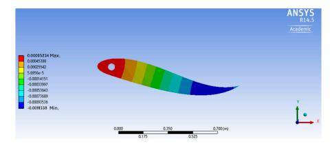
**Figure 4.** Deformation in case of  $E = 5 \times 10^4$  Pa at t = 2.1 s, Cl is reduced at this instant. Scale in y direction is scaled up.
