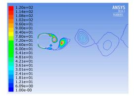
**Figure 7.** Distribution of vorticity for a circle at t = 15.4 s. Descending Cl.
