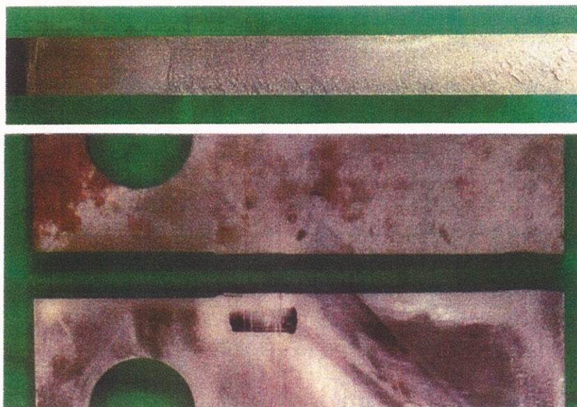
Fig.2.12 Fracture surface and pass after fracture toughness test (FTI-4, -159^{\circ}\text{C} )
