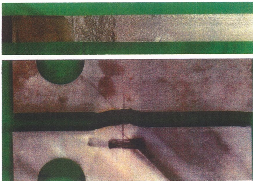
Fig.2.10 Fracture surface and pass after fracture toughness test (FTI-2, -144^{\circ}\text{C} )
