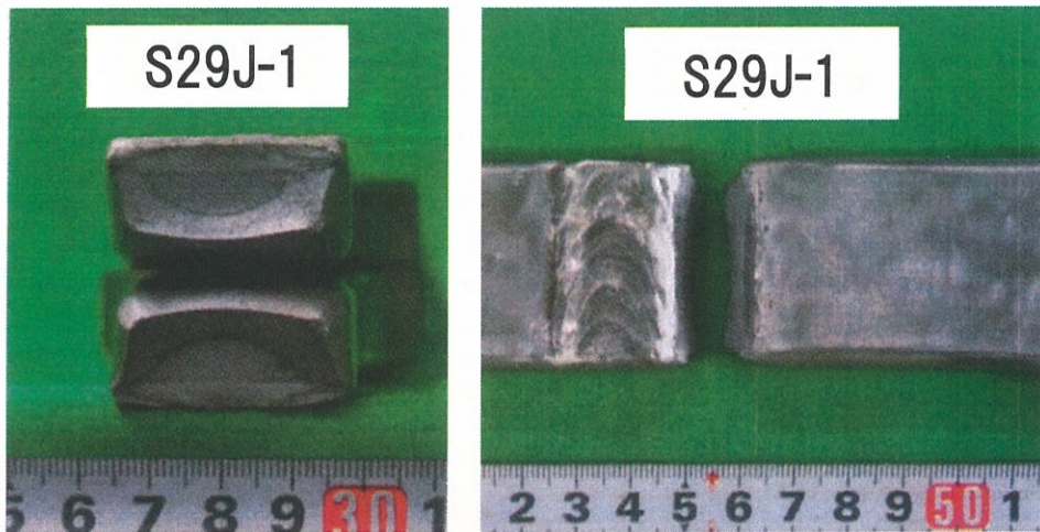
Fig.4 5 Fracture surface and pass after fatigue test [SUS329J3L-clad steel plate, As-welded S29J-1, 350N/mm 2 , 3.15 × 10 5 cycles]
