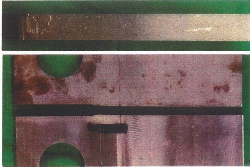
Fig.2.13 Fracture surface and pass after fracture toughness test (FTI-5, -173^{\circ}\text{C} )
