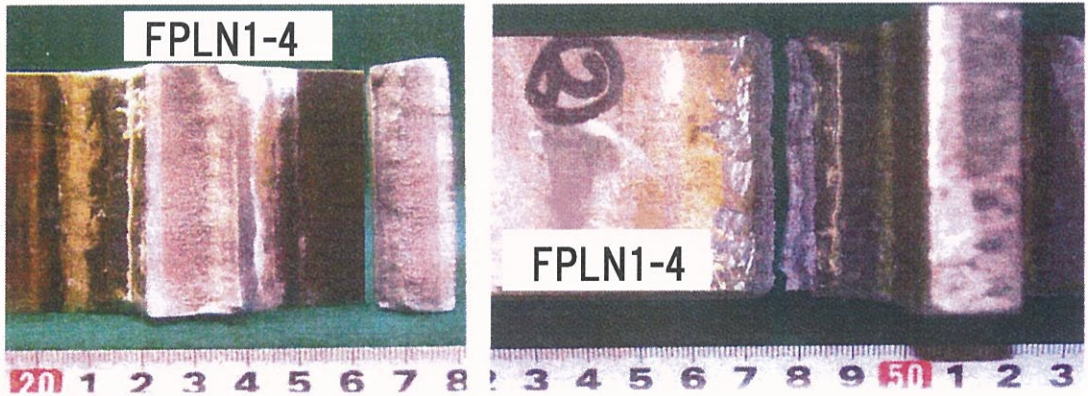
Fig.4.14 Fracture surface and pass after fatigue test [ SUS316L-clad + SUS329J3L-solid steel plate, As-welded, FPLN1-4, 250N/mm 2 , 1.66 \times 10^5 cycles ]
